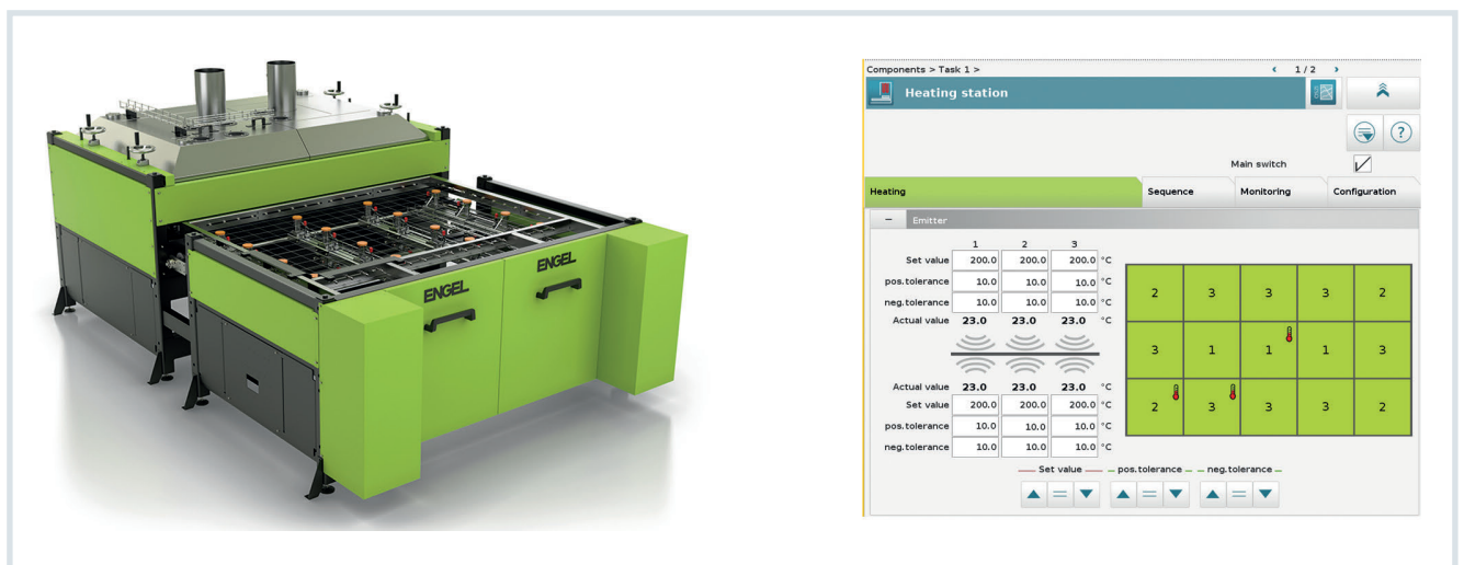
Fig. 2. A double-sided horizontal IR oven with 1100 x 600mm payload area: the radiators are combined into groups to allow for control on the basis of a specific temperature measurement © Engel
